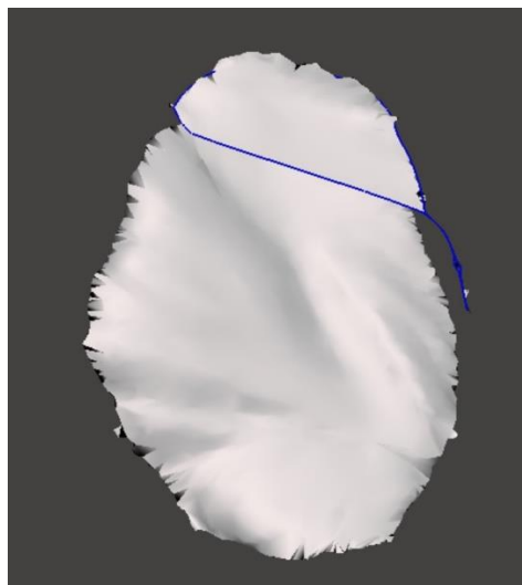
Figure 2: Inspector tool creates an extra layer over the defect in addition to filling the hole
