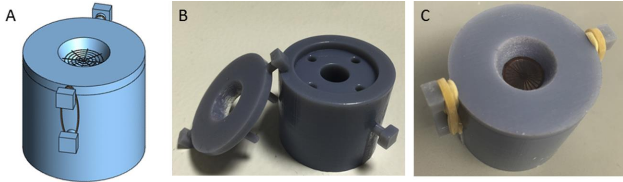
Fig. S1. Design and fabrication of sample holder for digital opto-electronic holography (DPOE) and laser Doppler vibrometry (LDV). (A) Customized 3D-printed holder was designed for use in DOEH and LDV experiments. The holder included a well for secure placement of a single TM composite graft or temporalis fascia. The cap was designed to completely cover the border region such that only the scaffold and collagen/fibrin infill were subject to acoustic testing. Dimensions for the base: inner hole diameter of 9 mm, well diameter of 25.5 mm, outer diameter of 35, inner well depth of 3 mm, and total length of 30 mm. The cap had the same inner and outer radii as the base with an extruded portion diameter of 25 mm, extruded portion length of 2.5 mm, and total length of 5.5 mm. (B) The holder was fabricated on an Objet Connex 500 printer (Stratasys, Minnesota, USA) with VeroBlue RGD840 rigid opaque material (Stratasys, Minnesota, USA). The design included four vertical pegs with a diameter of 2.6 mm to secure through gaps in the border region to restrict X and Y motion. It also included side pegs to secure the cap onto the base with elastics to restrict Z motion outside of the inner hole. (C) Placement of PDMS composite TM inside 3D-printed holder.
