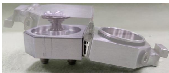
Figure S16. Image of the home-built transfer cell for the transport of the electrodes without exposure to air.
