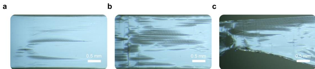
Figure S6: Optical images of 19 nm FS PS with tensile strain of a) 1.6%, b) 2.3%, and c) 3.5%. Gage length is 8 mm.
