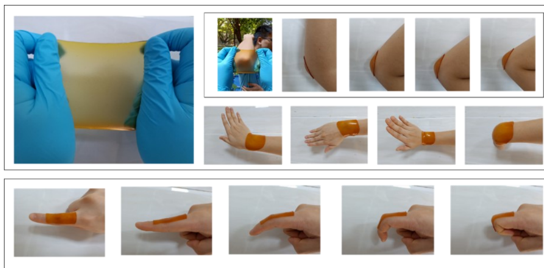
Figure S12. Digital photos of 10%BCD/PDA/PAM hydrogel adhered on elbow, dorsal side of wrist and finger with dynamic stretching along with the movement of joints.
