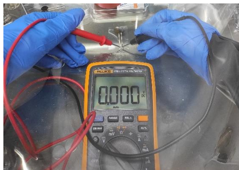
Fig. S4. OCV measurement of a drop-casted sample in Ar-filled glove box (RH ~0%).
