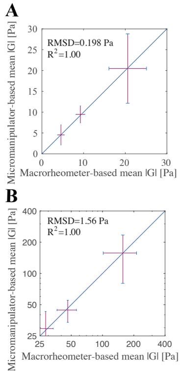
FIG. S4. Micromanipulator calibration against macrorheometry. (A) Micromanipulator 1 and (B) 2 compared against macrorheometer-based measurements, based on mean moduli  $|G|$ . Final volumetric force  $\hat{F}_{v,\text{probe}}$  conversion is based on the slope of 1.00 for the relationship (plotted). The errorbars show the measurement SDs.
