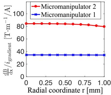
FIG. S1. Calibrated FEM simulation on magnetic-field gradient  $\frac{\partial B}{\partial x}$  dependence on radial position  $r$ , normalized by  $i_{\text{gradient}}$ . An axial coordinate of  $x=0$  is used.
