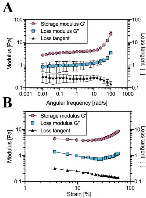
FIG. S5. Macrorheometer quantification of collagen type 1 at a concentration of  $c=1.0$  mg/mL.
