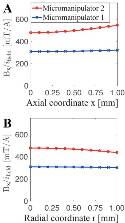
FIG. S2. Calibrated FEM simulation on magnetic field  $B_x$  dependence on (A) axial position  $x$  and (B) radial position  $r$ , both, normalized by  $i_{\text{field}}$ . (A) and (B) have a radial coordinate of  $r=0$ , and an axial coordinate of  $x=0$ , respectively.
