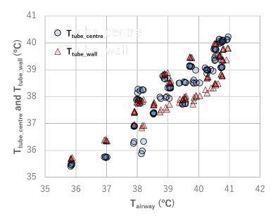
A representative scatter plot depicting the relationship between  $T_{airway}$ ,  $T_{tube\_centre}$  and  $T_{tube\_wall}$  with a representative setting (peak inspiratory pressure, 10 cmH<sub>2</sub>O; tracheal cuff, inflated; inspiratory time, 0.5 sec).
