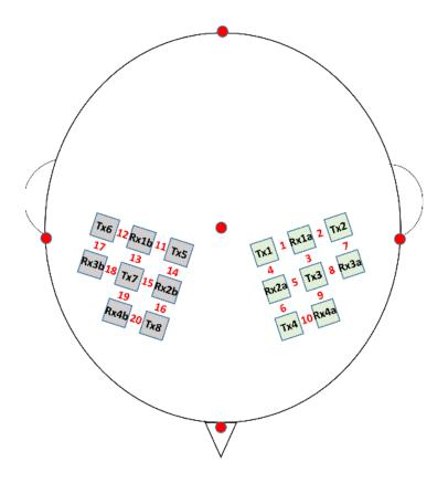
**Supplementary Figure 1.** Probe set arrangement of 20 channel fNIRS system: The red dots represent the reference points (nasion, Cz, inion and preauricular points) according to the 10-20 EEG system. Rx means receiver, Tx means transmitter. The red numbers indicate the measurement channel numbers. Tx3 refers to F3 (left hemisphere) and Tx7 refers to F4 (right hemisphere) of the EEG nomenclature.
