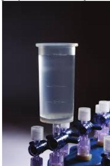
Figure 2. The PureYield™ Midi Binding Column is attached to a Vac Man vacuum manifold port.
