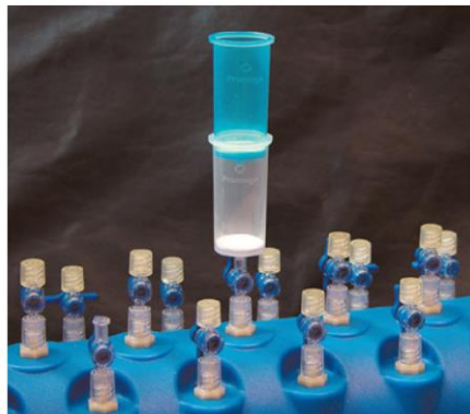
Figure1. The blue clearing column inserted into the white binding column. The two columns sit on a vacuum manifold port.
