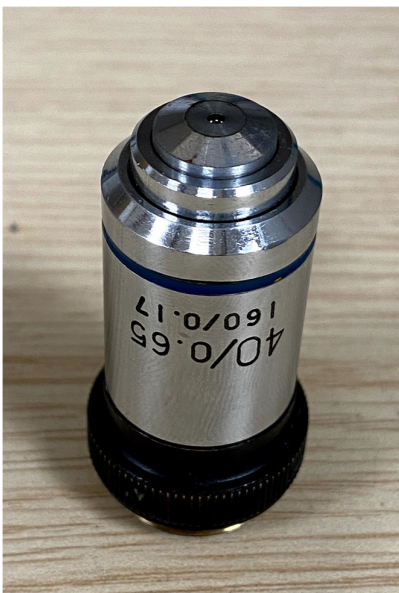
Fig. R1: Microscope objective to de-magnify the projection image in the object simulation setup.
