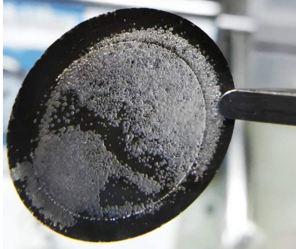
Supplementary Fig. 29 Optical photo of Na deposition on Sn-coated separator with 4 mAh/cm 2 at 1 mA/cm 2 .
