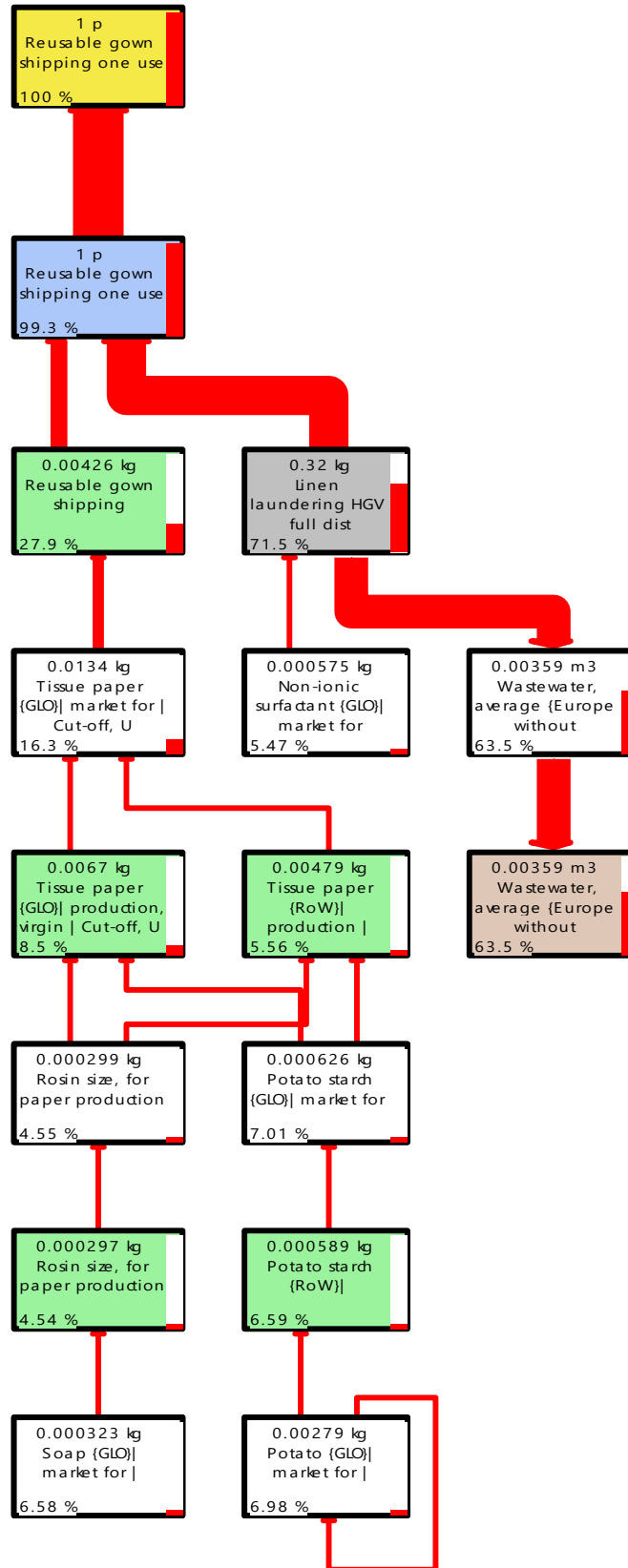
Supplementary Figure 11: Network diagram for a reusable gown showing marine eutrophication impact drivers (5% cut-off)
