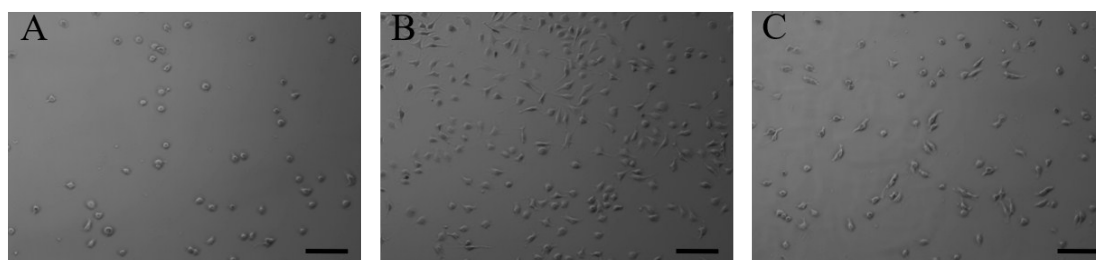
Figure S8. MSCs adhesion behaviors on surface 1 (A), surface 2 (B), and surface 3 (C). For all of the surfaces, the adhesion time is 3 h. Scale bar is 100 \mu\text{m} .
