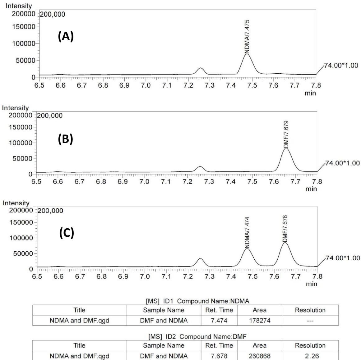
Figure S1. The representative chromatograms of (a) spiked NDMA ( $m/z$  74), (b) spiked DMF ( $^{15}\text{N}$  isotopic ion at  $m/z$  74) and (c) co-spiked between NDMA and DMF in losartan
