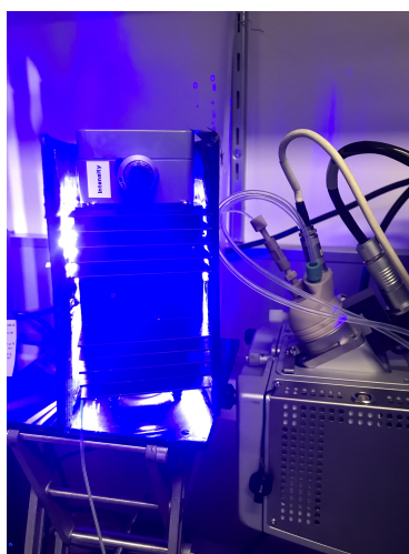
Figure S9: Schematic representation of the real-time photoreaction screening platform using the charge tagged palladacycle 4 . The progress of the reaction and intermediates were monitored at 100 \mu M concentration in acetonitrile on the positive-ion mode with the 448 nm (15 W) blue LED photoreactor.
