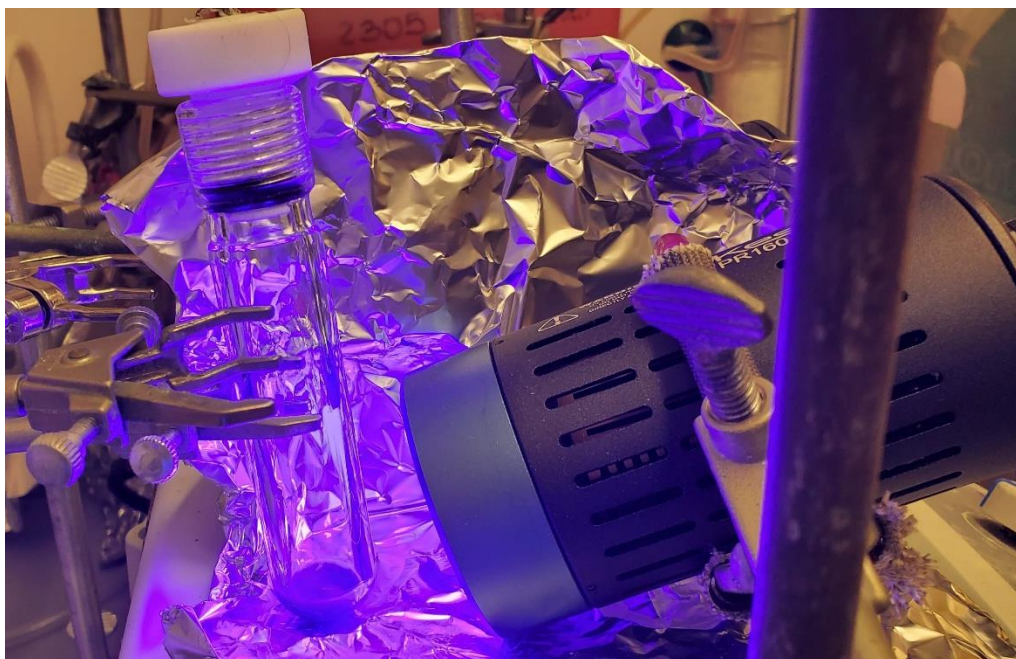
Pressure tube and Kessil lights for aminocarbonylation (Swagelok adapter not pictured)
