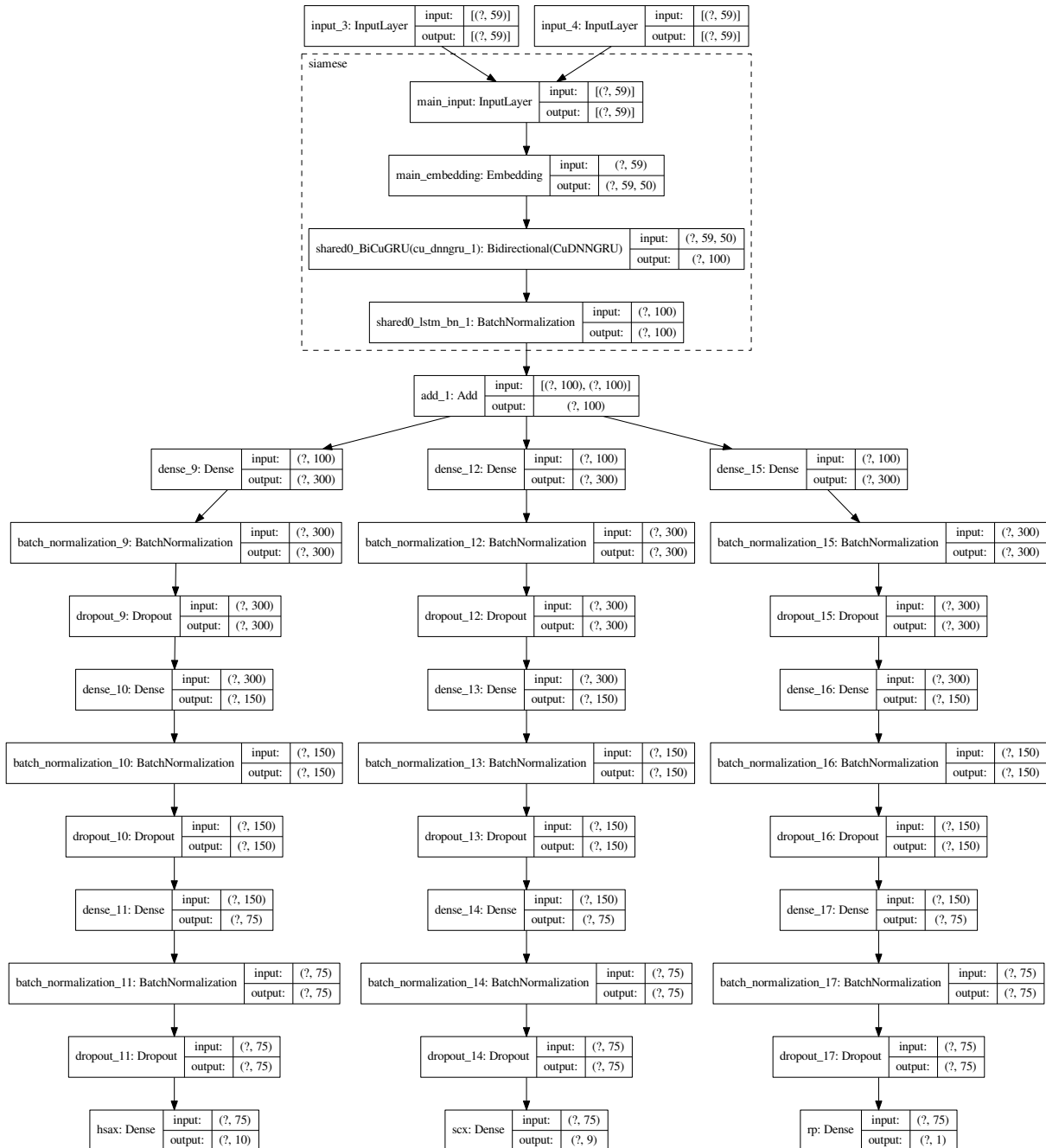
Supplementary Figure 1: Example parameterization of xiRT. Dashed box represents the Siamese network part. Boxes represent individual layers with their names, input and output dimensions. Question marks represent the unknown batch-size at compilation time of the network.
