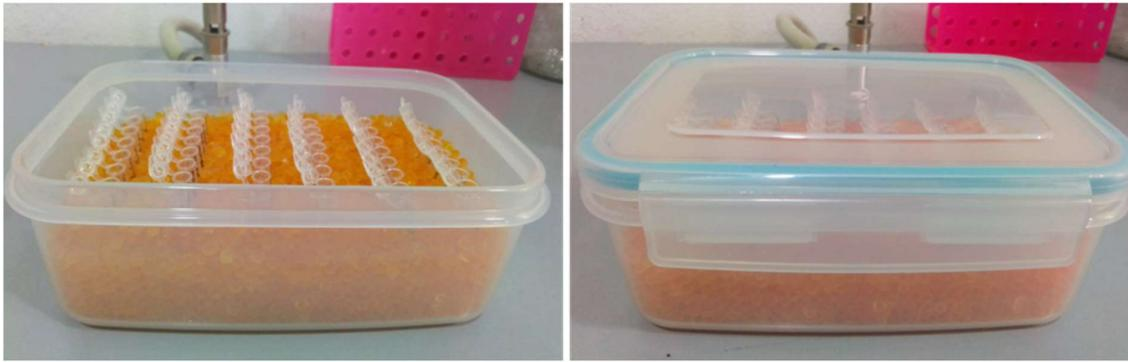
**S2 Fig. Sample disposition in the air-tight container for the preparation of evaporated OpenVent cellular reagents.**
