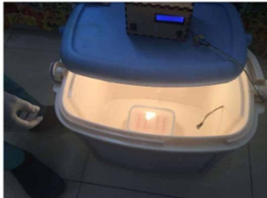
**S3 Fig. DIY incubator built from locally sourced materials.** Top panel: Arduino scheme to control the DIY bioreactor. Bottom panel: DIY incubator final assembly.
