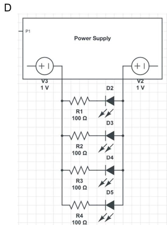
**S14 Fig. Design and construction of fluorescence visualization box.** (A) Visualization box with 3D printed tube chamber and LED circuit board. (B) Image showing placement of LAMP-OSD tubes inside the visualization box. (C) Top view of the LED circuit board. (D) Circuit design. (E) Bottom view of the circuit board. Detail instructions available at <https://github.com/Jose-4625/LAMP-BOX-ECO/tree/master/VisBox>.
