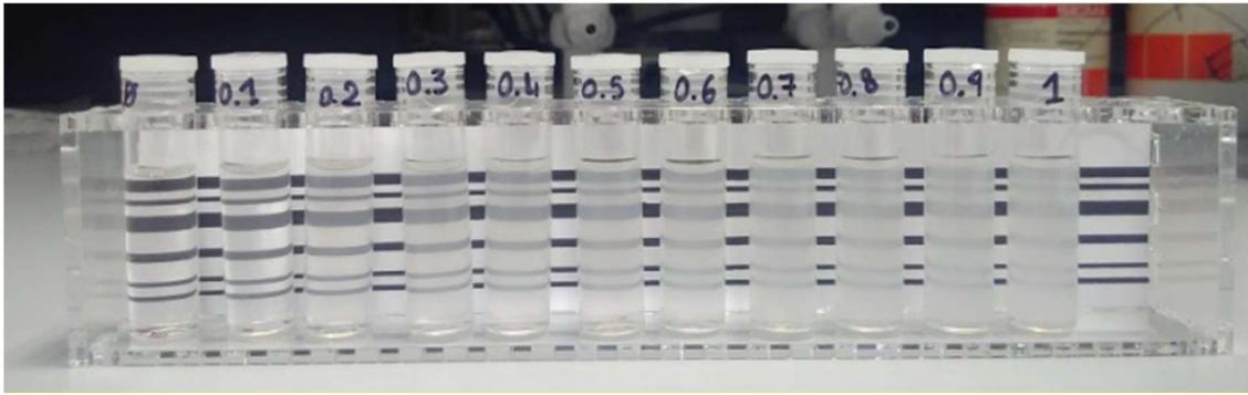
**S1 Fig. McFarland turbidity standards.** The standards are visualized from the side on a test tube rack against a drawn black and white pattern. The sample to be tested must be aliquoted in the same type of tube used for the standards.
