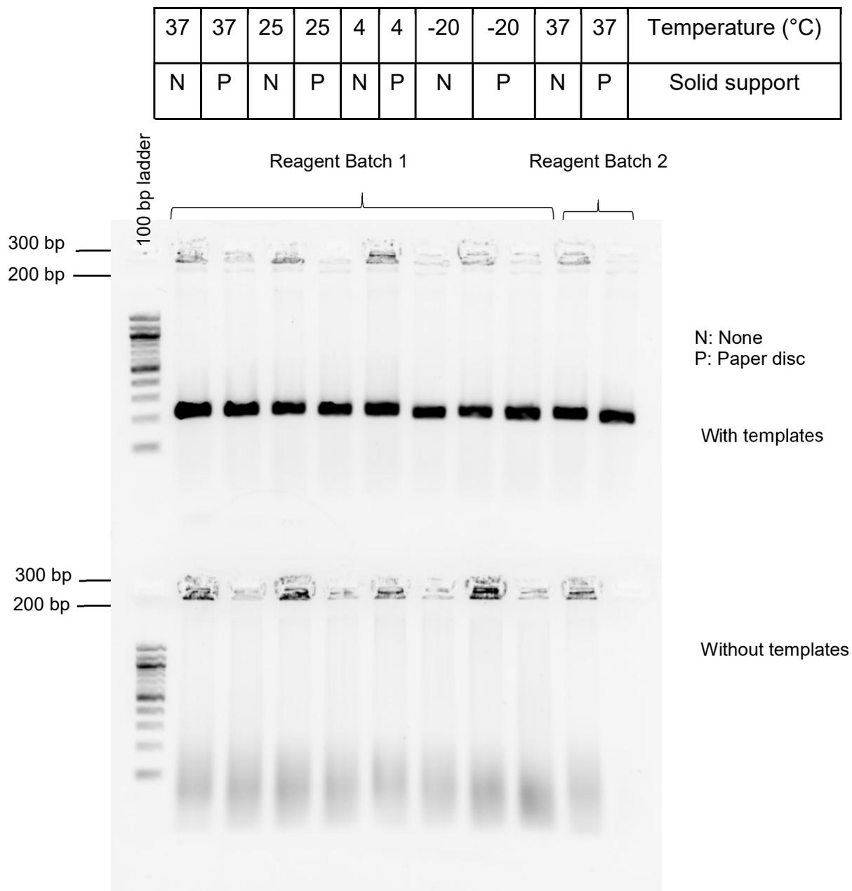
**S10 Fig. Endpoint PCR using Taq DNA polymerase cellular reagents dried in the presence or absence of desiccant.**
