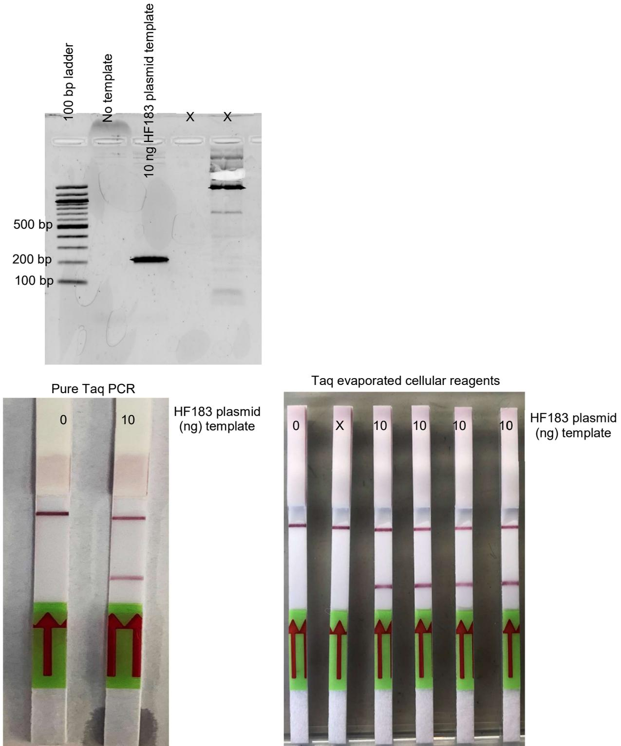
**Fig 9.** LAMP-OSD based molecular testing kit using Bst-LF evaporated cellular reagents. 80,000 (+) or 0 (--) copies of HF183 plasmid templates were amplified using HF183 LAMP-OSD assays operated with either Bst-LF cellular reagents (CR) or with pure Bst 2.0 enzymes. Endpoint image of OSD fluorescence was taken using a ChemiDoc camera (Bio-Rad, Hercules, CA, USA). Lateral flow dipsticks inside Ustar cartridges were imaged using a smartphone camera.
