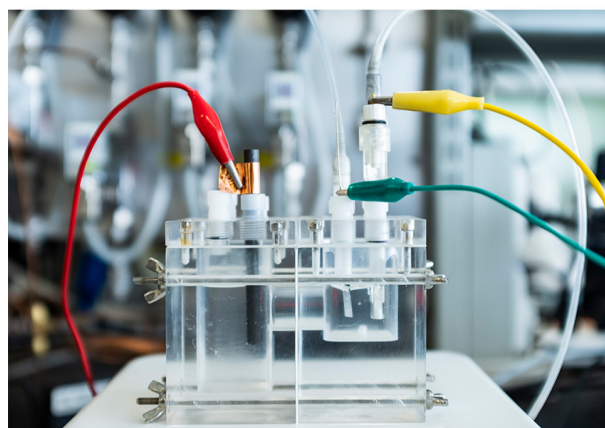
Supplementary Figure 1. Image of the three-electrode H-cell employed for CO electrolysis study.
