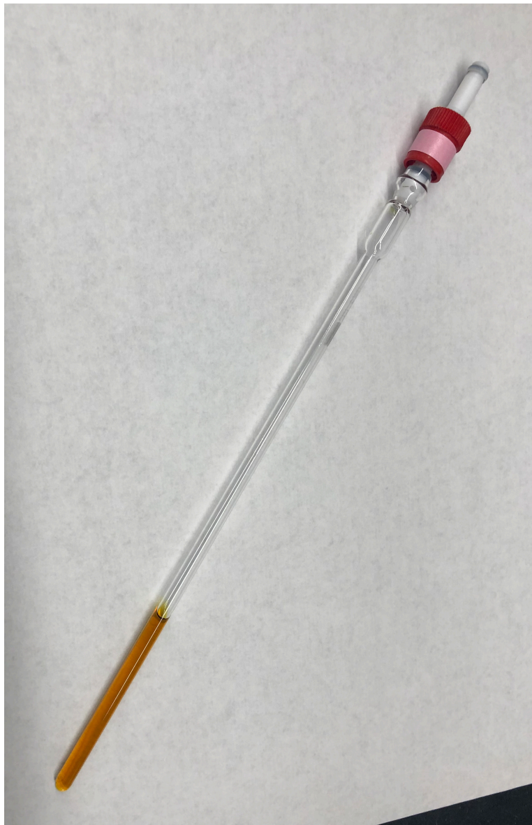
Figure SI-8. J-Young-style NMR tube used in mechanistic spectroscopy experiments
