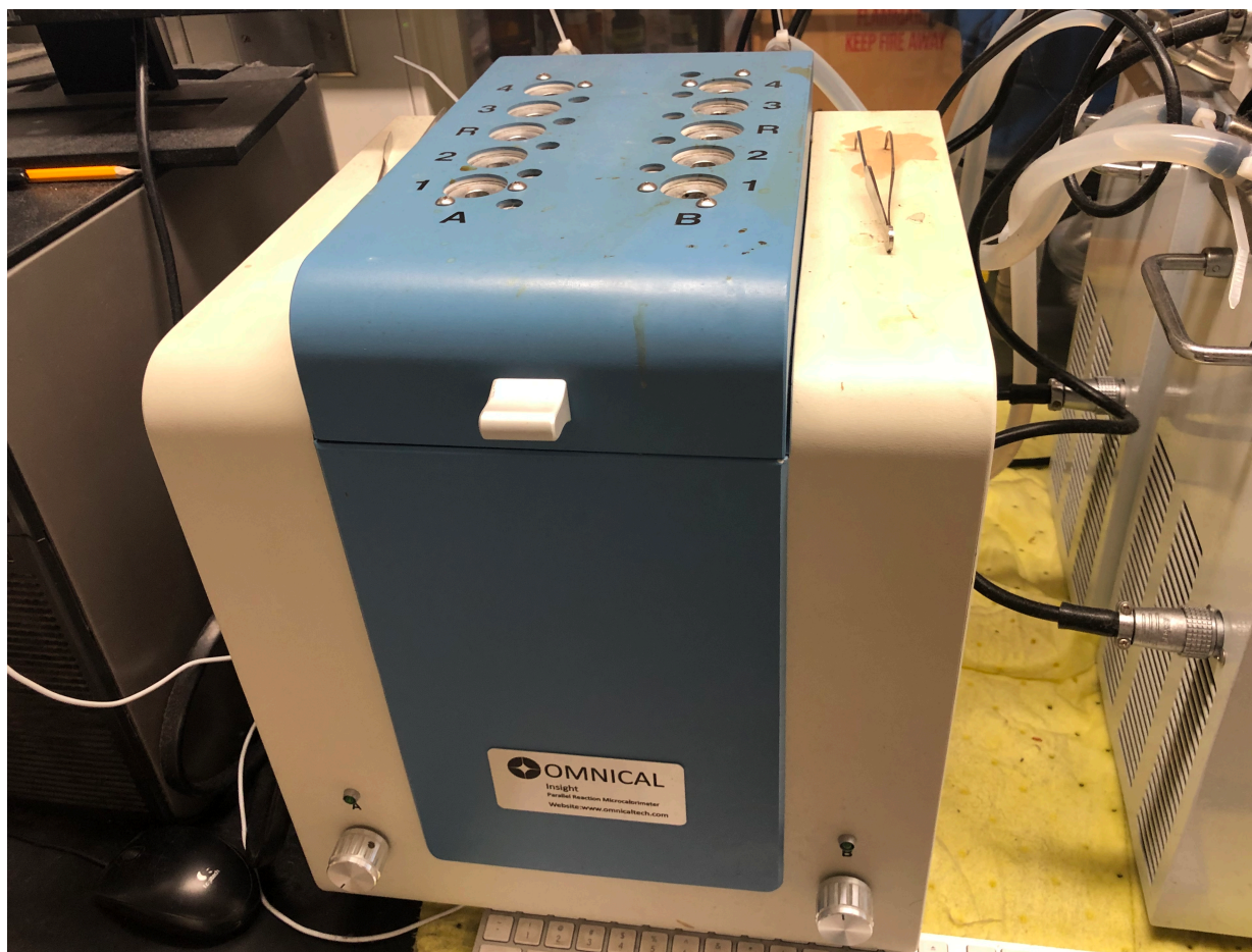
Figure SI-1. Omnical Insight Parallel Reaction Calorimeter used in kinetics experiments.
