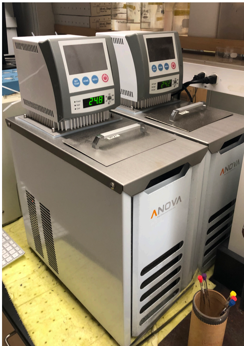
Figure SI-2. Anova constant-temperature oil-recirculating baths associated with the calorimeter.
