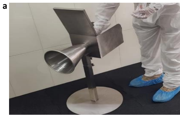
a Metal search stand showing the cone and sample holder compartment
