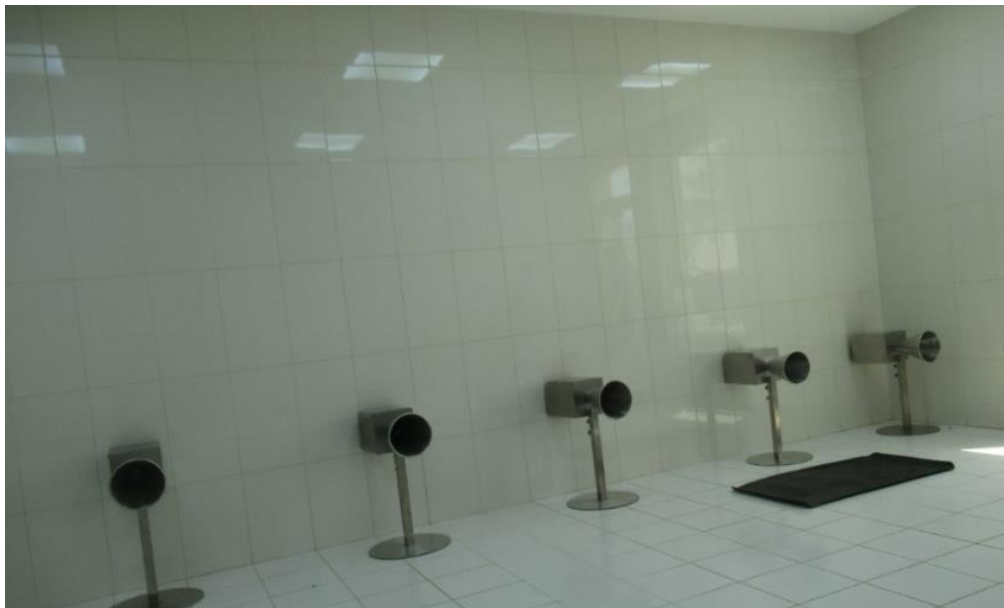
Five metal search stands are shown in the training room. Each stand has a sniffing cone and a specimen holder compartment right behind it
