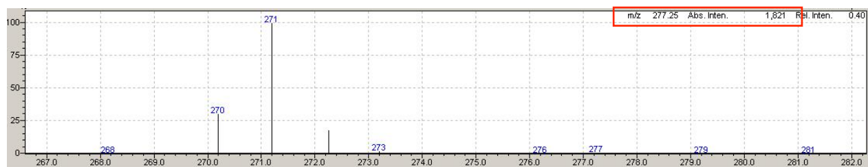
Figure S20. Zoomed GC and MS traces of borylative exchange of 5d with HB(pin- d 6 ) in the absence of 1 (reaction B ).
