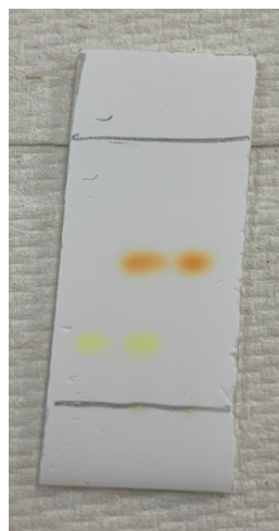
Figure S4. TLC analysis (before and after KMnO 4 stained) after stirring at 23 °C for 10 min.
