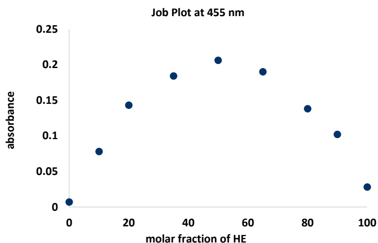
Figure S3: Job plot of the EDA complex (0.2 M total concentration in DMA) between Hantzsch-ester HE and N -cyclohexyl-hydroxyphthalimide-ester ( 2 ) recorded at 455 nm.
