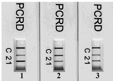
Fig. S1. RPA assay optimization for primer and probe concentration. Multiplex RPA reactions were performed following the provider instructions. Clavibacter -specific primer/probe concentrations were evaluated against Cn -specific primer/probe set. 1) low ( Cn 1.2 \mu L/1.4 \mu L; Clavibacter 0.8 \mu L /0.6 \mu L); 2) equal ( Cn 1.2 \mu L/0.8 \mu L; Clavibacter 1.2 \mu L/0.8 \mu L); and 3) high ( Cn 1.5 \mu L/0.9 \mu L; Clavibacter 1.0 \mu L/0.6 \mu L).
