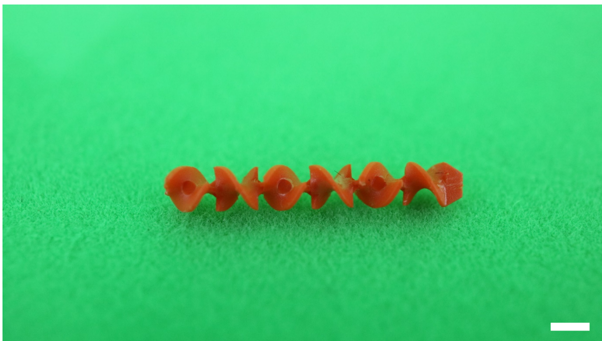
Figure S5. Static mixer. Picture of the mixing element used in this study. Scale bar 2 mm.
