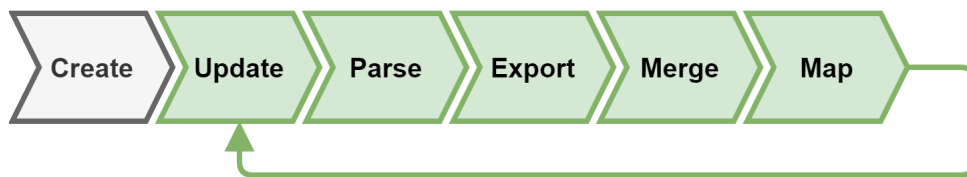
Figure 2: The program flow of BioDWH2 from the creation of a workspace to the final merged and mapped graph database. When new data is available, the process starts over at the update step.
