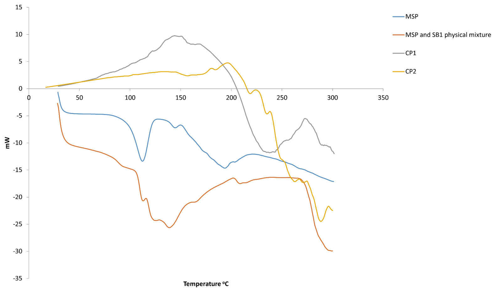
Figure S10. Differential scanning calorimetric (DSC) thermograms of MSP, MSP: SB1 physical mixture, CP1 and CP2.
