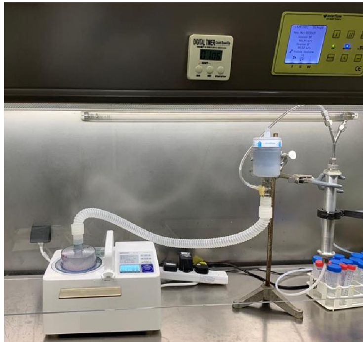
Supplementary Figure 1. Laboratory set up of the particle aerosolization system used for dispersing virus onto filters.
