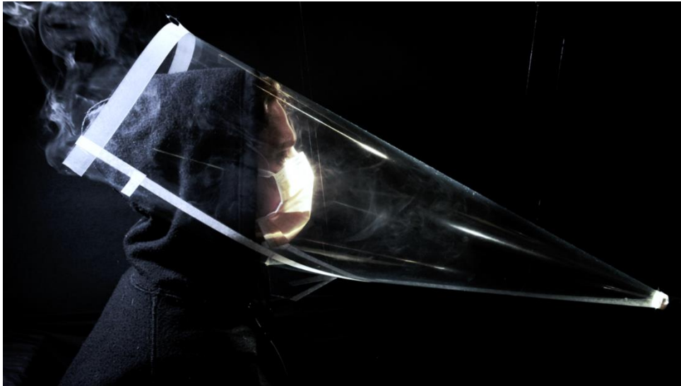
S3.9 - Talking demonstrated deflection around the mask, which is subsequently captured on an upward thermal plume of body heat and carried upwards and out of the cone (2:19:27*).
