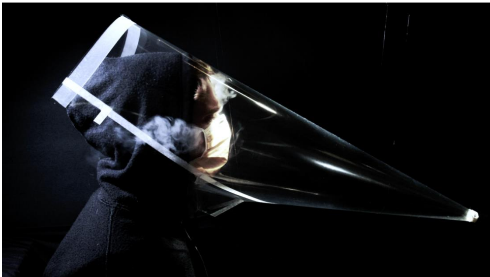
S3.10 – Considerable quantities of high velocity exhaled gas is observed deflecting backwards following a cough (2:42:10*)
