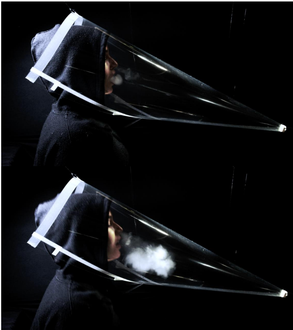
S3.5 - High efficiency of particle capture during open limb NIPPV-S breathing IPAP/EPAP pressure 25/10 cmH 2 O. Two exhalation plumes visible, the first via anti-asphyxia valve near to mask, the second via the open expiratory port towards bottom of picture (3:41:08*)
