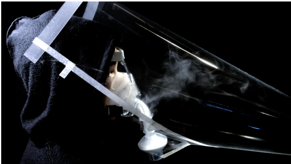
S3.4 - High efficiency of particle capture during closed limb NIPPV-D IPAP/EPAP pressure 25/10 cmH 2 O. Note leakage via the facemask anti-asphyxia valve. (3:08:17*)
