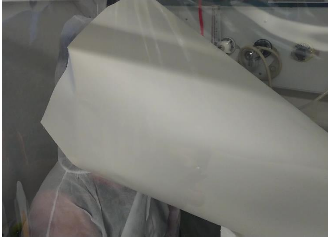
Figure S3.1 – Photograph taken of a subject within the aerosol measuring chamber during the sampling protocol. Note, backwall made of electret material, Perspex walls, experimental sampling cone composed of electrically conductive aluminium coated cardboard, polypropene hooded jacket worn by subject.
