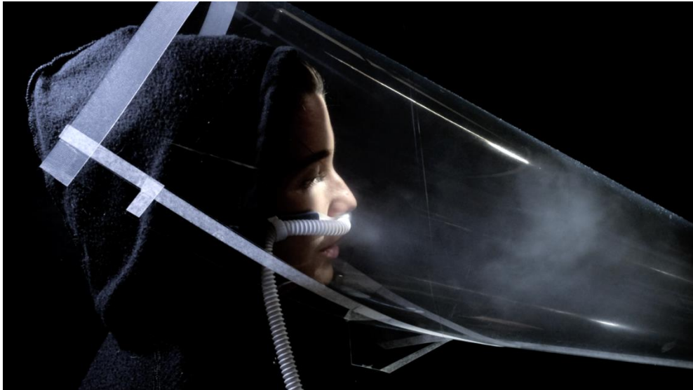
S3.3 - High efficiency of particle capture during breathing receiving HFNO at 60\text{L}\cdot\text{min}^{-1} flow. Despite high exhaled gas dispersal due to HFNO flow, the large cone and high sample rate sampling maintains high sampling efficiency (2:55:05*).
