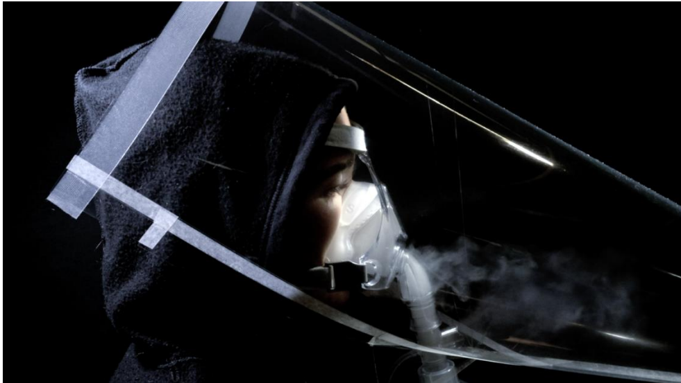
S3.5 - High efficiency of particle capture during open limb NIPPV-S breathing IPAP/EPAP pressure 25/10 cmH 2 O. Two exhalation plumes visible, the first via anti-asphyxia valve near to mask, the second via the open expiratory port towards bottom of picture (3:41:08*)
