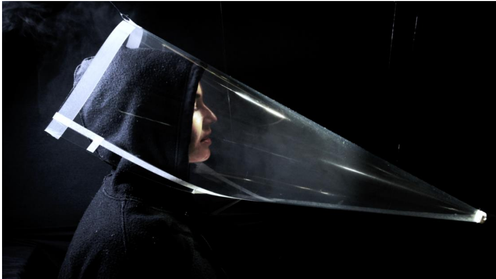
S3.7 – Image from 4 seconds following a cough. High velocity gas is observed to be deflected backwards and an unquantified proportion is ejected from the rear of the cone. (1:49:06*)
