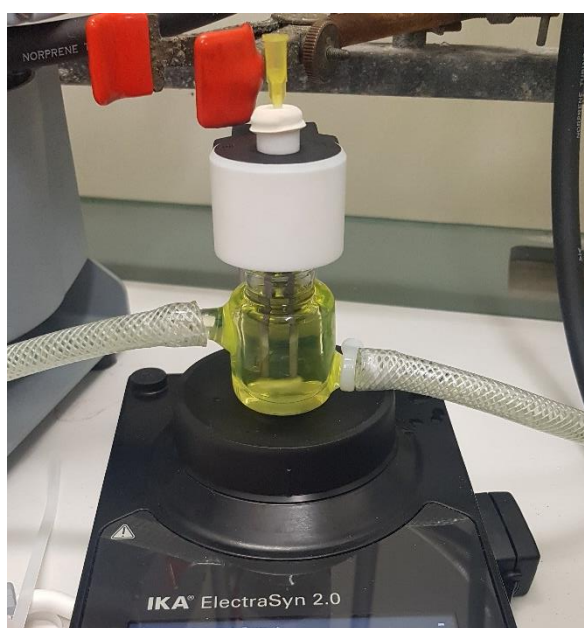
Picture 2: Home-made cell to control the temperature.
