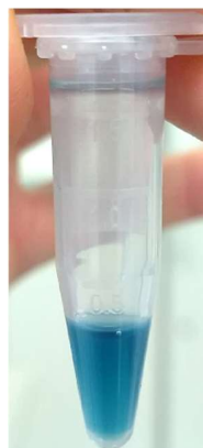
Figure S6. Reaction mixture (250 \mu L total volume) performed in a 1.5 mL Eppendorf tube. The blue colour results from the dissociation of Bromothymol blue in solutions that are more basic.
