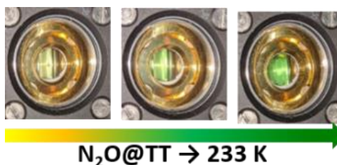
Figure S16: Observed color change during reaction with nitrous oxide and increasing the temperature from 193 K up to 233 K. After addition of \text{N}_2\text{O} at 193 K the color of the precursor complex 1a and 1b changed from yellow to pale yellow. Upon increasing the temperature, the characteristic green can be observed.
