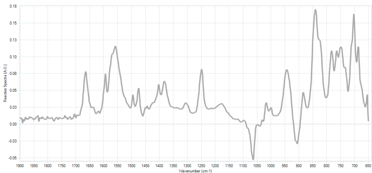
Figure S7. ReactIR spectrum of a 0.17 M solution of 2-((3-chlorophenyl)(phenyl)methyl)- N -methylbenzamide ( 4g ) (0.25 mmol) in THF plus 0.2 mL of 1 M KHMDS. Note – analysed solution is colourless.
