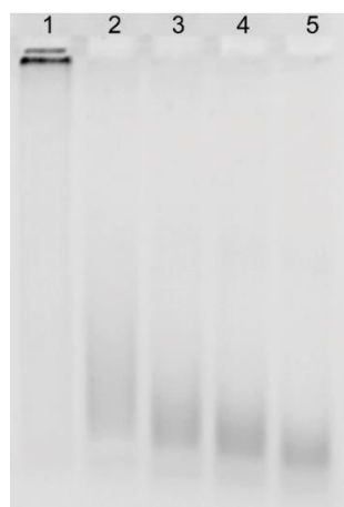
Figure S5. 1% agarose gel to trace ultrasound treatment of pTBA 15 for different time periods. From lane 1-5: 0, 30, 60, 180, and 300 s.
