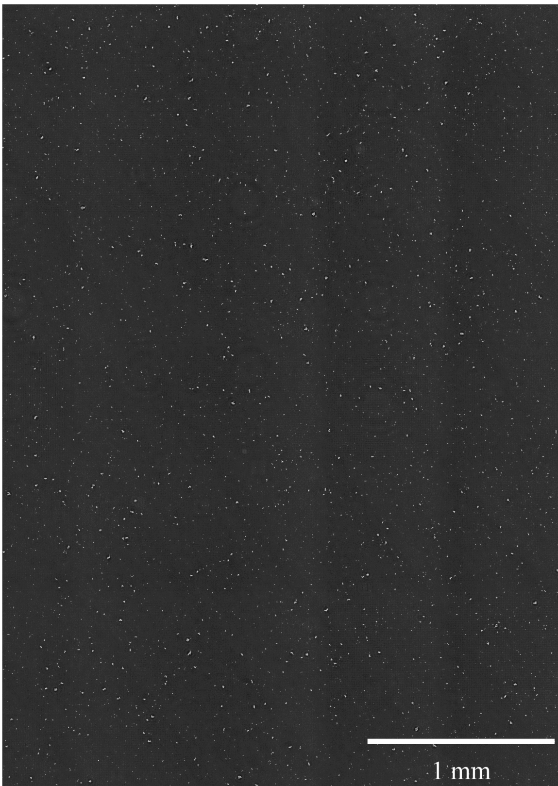
Figure S7: Full FOV reconstruction for a sample containing 2 \mu\text{g}/\text{mL} of NA and 0.01% 2- \mu\text{m} B-beads in PBST. This sample has 18268 2- \mu\text{m} B-beads exhibiting a bound ratio of 80.39%.
