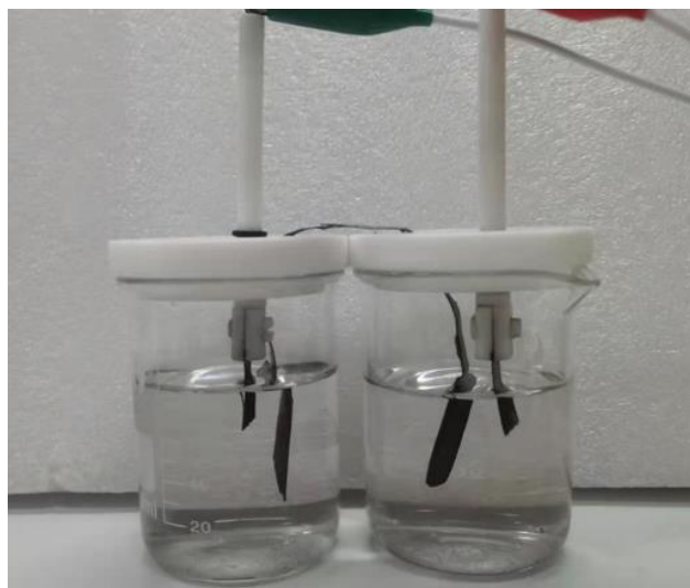
Supplementary Figure 19: Photograph of the conventional decoupled electrolyzer using \text{NiOOH}/\text{Ni}(\text{OH})_2 redox couple.
