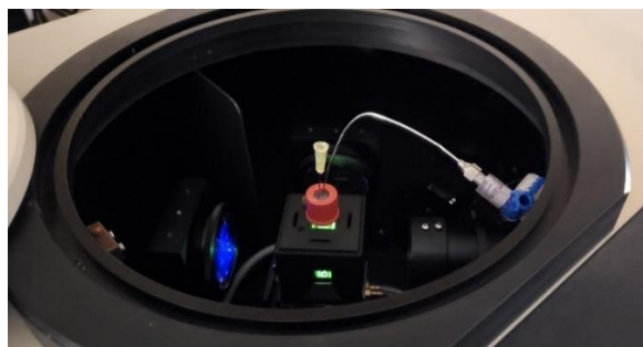
Figure 5. The photoredox reaction set-up. The reaction mixture was irradiated at 406 nm under an atmosphere of Ar (g) at 23 °C.
