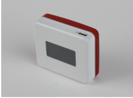
Fig. S1. Ultrasound-on-chip patch prototype. A functioning prototype of an ultrasound “patch,” build using Ultrasound-on-Chip technology.
