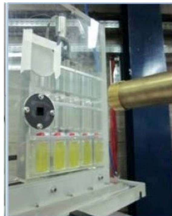
Supplementary Figure 1: Set-up for cellular irradiation at INFN-LNS. On the right, the CATANA proton beam line is shown, where A. Kapton window; B. Box encapsulating the energy modulator wheel ( B1 ) and range shifter ( B2 ); C. Monitor chambers; D. The MOPI detector for online beam profile monitoring; E. End-of-line collimator. The two pictures (centre and left) show the mechatronic holder flask system, which allows to control remotely the movement of the sample holder in front of the beam collimator
