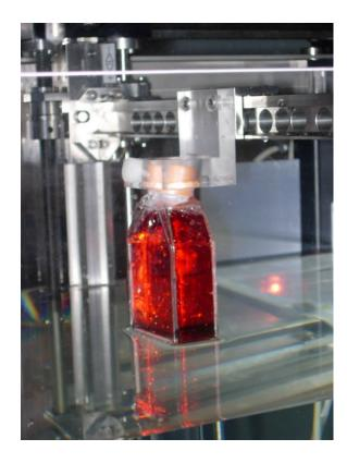
**Supplementary Figure 2.** Set-up for cellular irradiation used at the high-energy CNAO protontherapy beamline. On the left, next to the beam exit is shown the water tank where tissue culture flasks were placed for radiation exposure at different depths corresponding to various positions along the SOBP (see main text, Section see section Clinical High-Energy Proton Beamline). The picture on the right shows in detail a flask before being submerged held on to a motorized arm.
