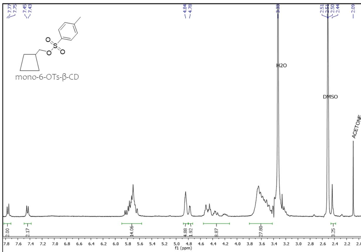
**Figure S4. <sup>1</sup>H NMR of mono-6-OTs-β-CD.** Mono-6-OTs-β-CD chemical structure was verified using <sup>1</sup>H NMR in DMSO-d<sub>6</sub>. δ = 7.76 (d, 2H), 7.44 (d, 2H), 5.89-5.56 (m, 14H), 4.84 (s, 5H), 4.78 (s, 2H), 4.12-4.55 (m, 9H), 3.8-3.42 (m, 28H), 3.41-3.06 (m, overlaps with H<sub>2</sub>O), 2.42 (s, 3H). Other peaks are a result of solvents used during reaction or DMSO-d<sub>6</sub> and are noted on the spectrum.
