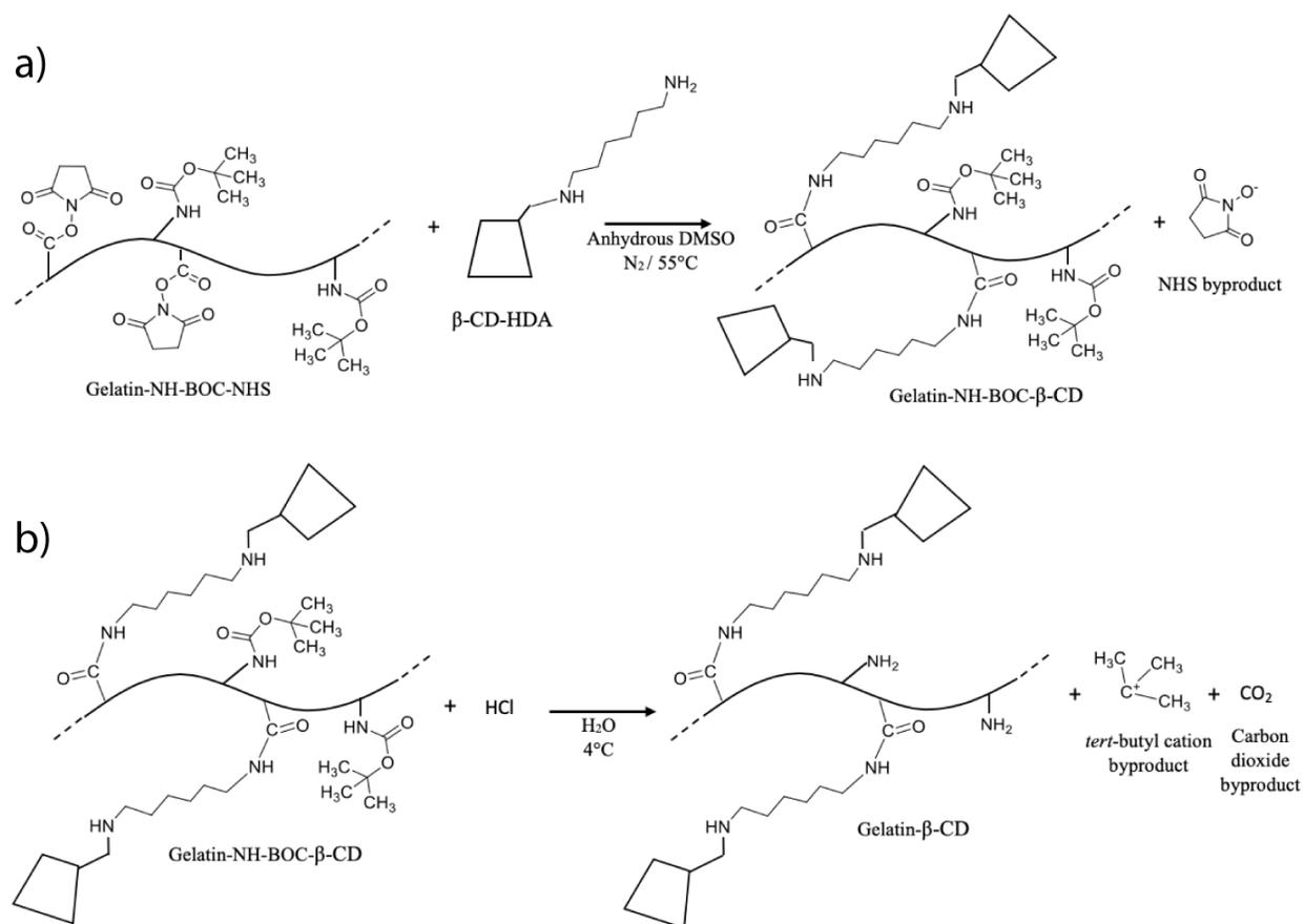
**Figure S6. Synthesis of Gel-CD.** Gel-NHS-Boc is reacted with CD-HDA under dry DMSO and N<sub>2</sub> conditions. An amide bond is formed between the activated carboxylic acid on the gelatin backbone and the primary amine of CD-HDA. Boc deprotection with mild acid yields the final Gel-CD species.
