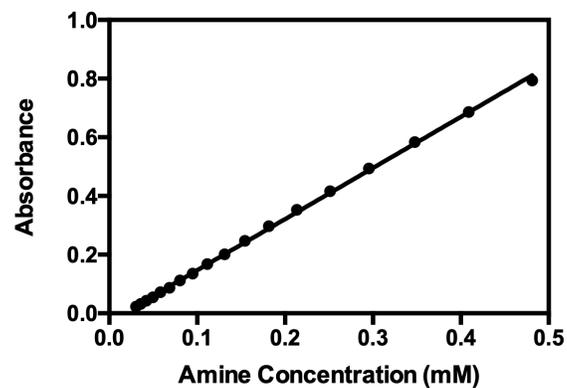
**Figure S7. Calibration curve for primary amine concentration.** Calibration curve to determine amine concentration in modified and unmodified gelatin was prepared using glycine standards in increasing concentrations and under identical conditions and OPA stock solution. A linear correlation with  $R^2 = 0.9993$  was observed, following the Beer-Lambert law.
