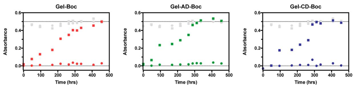
**Figure S8. Deprotection of modified gelatin.** Amine content of unmodified gelatin (grey), Gel-Boc (red), Gel-AD-Boc (green), and Gel-CD-Boc (blue) was determined a function of time for untreated samples (circles) and those treated with 0.5% v/v HCl 12M (squares), as measured using the OPA reagent with an assay absorbance of 340 nm.
