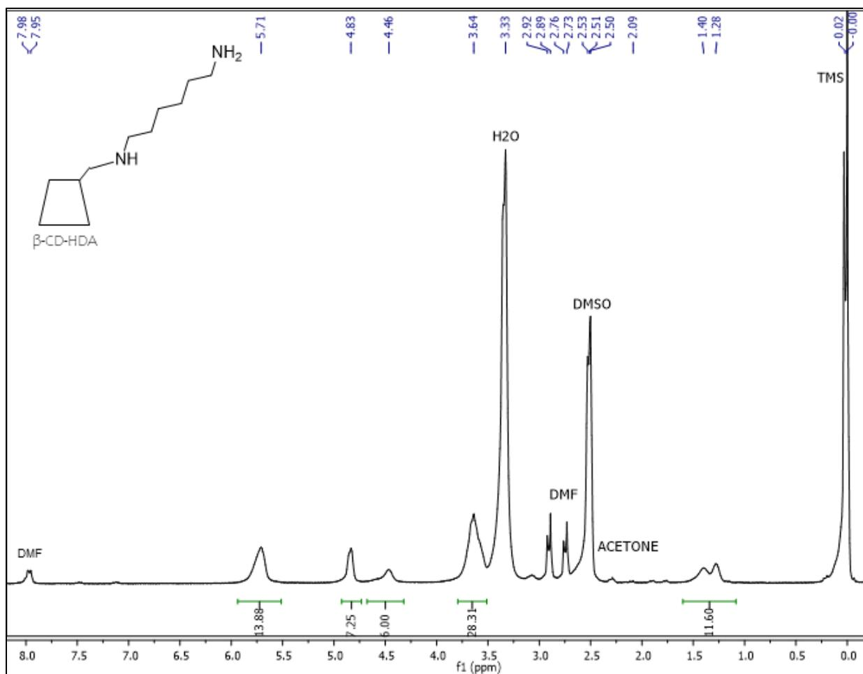
**Figure S5.  $^1\text{H}$  NMR of CD-HDA.** CD-HDA chemical structure was verified using  $^1\text{H}$  NMR in DMSO- $d_6$ .  $\delta = 5.71$  (br s, 14H), 4.83 (br s, 7H), 4.46 (br s, 6H), 3.79-3.5 (m, 28H), 3.5-3.17 (m, overlaps with  $\text{H}_2\text{O}$ ), 1.6-1.08 (m, 12H). Other peaks are a result of solvents used during reaction or DMSO- $d_6$  and are noted on the spectrum.
