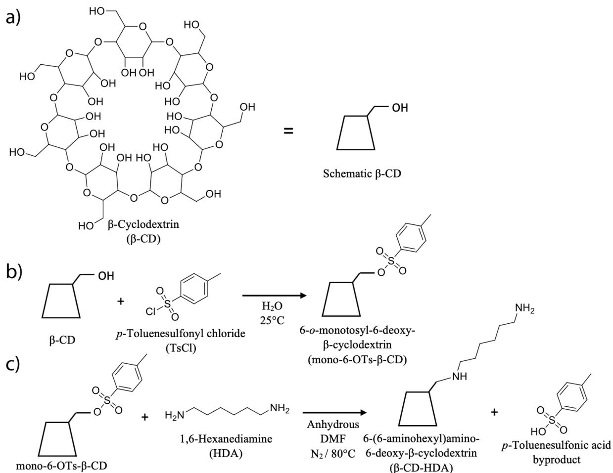
**Figure S3. Synthesis of CD-HDA.** (a) Schematic representation of  $\beta$ -Cyclodextrin (CD). (b) First step of alcohol activation using TsCl. Single tosylation was achieved by dropwise addition of TsCl to a basic aqueous solution containing CD. (c) Excess of HDA was introduced to the dry mono-6-OTs- $\beta$ -CD under anhydrous conditions for overnight reaction at 80 °C. Final product CD-HDA was achieved as a white powder.
