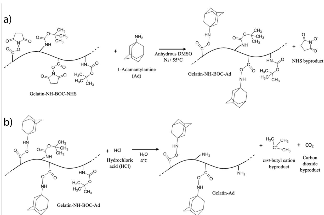
**Figure S2. Synthesis of Gel-AD.** Gel-NHS-Boc is reacted with 1-adamantylamine (AD) under dry DMSO and N<sub>2</sub> conditions. An amide bond is formed between the activated carboxylic acid on the gelatin backbone and the primary amine of AD. Boc deprotection with mild acid yields the final Gel-AD species.
