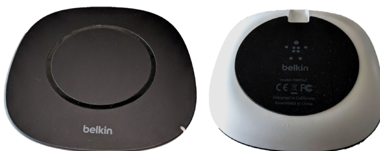
Figure 7. Top and Bottom view of a wireless charger base
