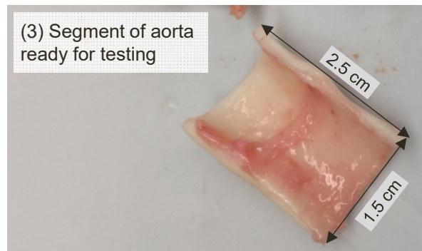
Supplementary Figure 2. Preparation of a sample of bovine aorta for electroadhesion experiments. (1) As received, in the “raw” state, the aorta is encased in fat, and connected to other tissues. (2) The aorta is removed from the surrounding tissues and the fat encasings. (3) A segment of the aorta is cut to the desired size, comparable to the size of a gel segment. This is used for the electroadhesion experiments.
