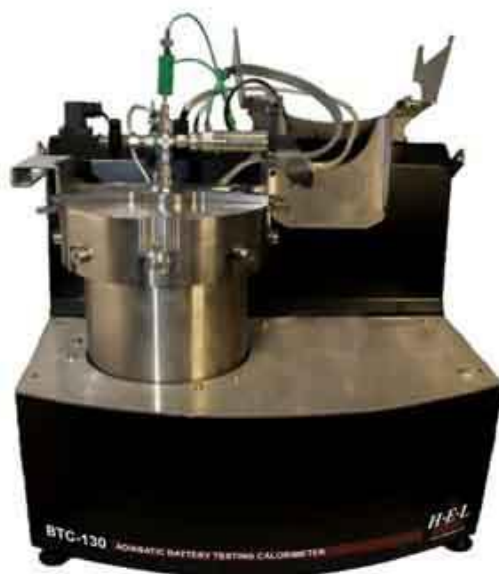
Figure S4 The photographs of ARC (BTC130, HEL) for thermal runaway study of battery materials.
