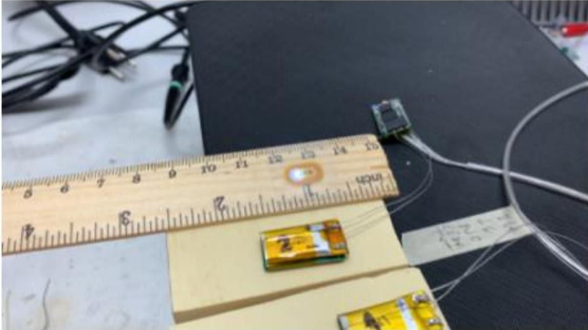
**Supplementary Video S1: Wireless Recharging.** The video demonstrates a deconstructed spinal stimulation circuit with an inductive charging coil placed on top of an inductive charging pad designed to fit over the bottom of a rat housing chamber. A ruler with an LED powered by an inductive charging coil is also visualized over the charging field. The light demonstrates areas where the battery is effectively able to charge over the surface of the charging pad.
