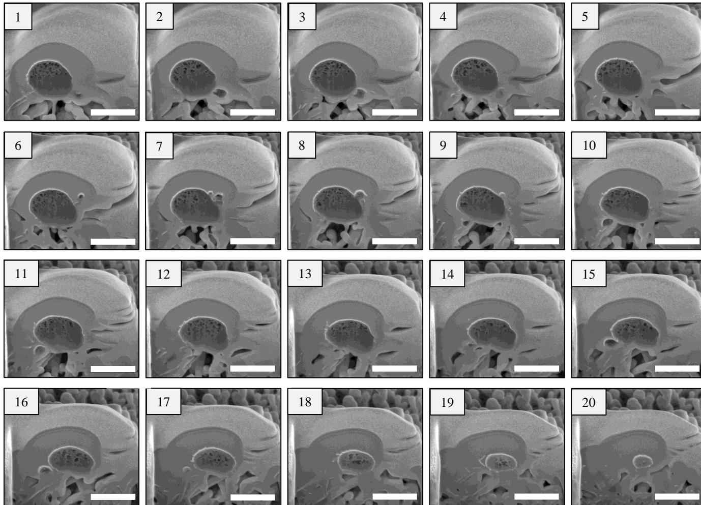
**Supplementary Figure 2. Slice and view focused ion beam milling of *E. coli* with platinum deposition.** FIB-SEM was used to generate sequential 30 nm cross sections through *E. coli* with a protective platinum coating. The milling interface of 20 serial sections is shown. Scale bar: 500 nm. Related to Figure 2.
