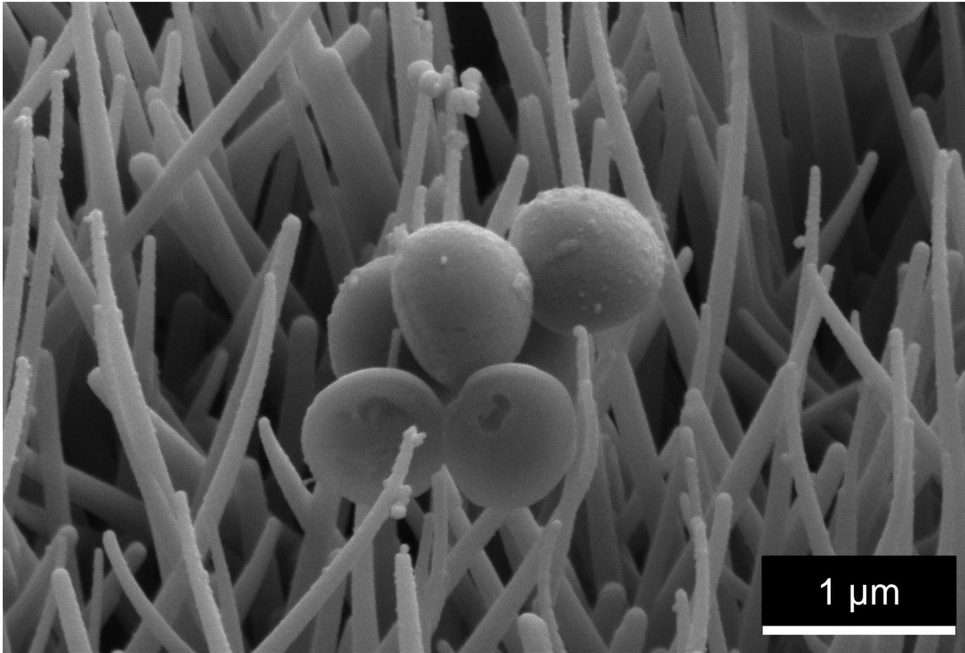
**Supplementary Figure 5. Evidence for *S. aureus* cell impedance induced by TO-NS-Long surface.** Representative scanning electron micrographs of *S. aureus* impeded by TiO<sub>2</sub> nanostructures on TO-NS-Long surfaces. Cross sections through *S. aureus* cells show no evidence of envelope deformation or penetration, but clearly show that *S. aureus* cells have adhered between the nanostructures. Related to Figures 8-9.
