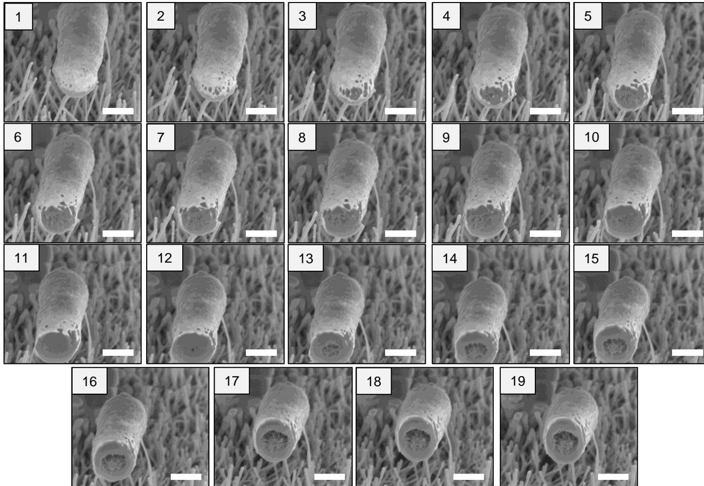
**Supplementary Figure 1. Slice and view focused ion beam milling of *E. coli* without platinum deposition.** FIB-SEM was used to generate sequential 30 nm cross sections through *E. coli* without a protective platinum coating. The milling interface of 19 serial sections is shown. Scale bar: 500 nm. Related to Figure 2.
