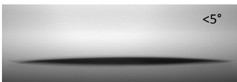
Figure s2: Glass slides were used as the base of the avidin and APTES treated slides. They had a contact angle of <5^\circ . The contact angle after each treatment step is shown in Figures 3 and s3.
